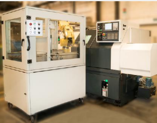
Robot Interface with Machine & Carousel
