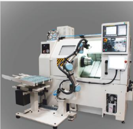
Stacker Type- Machine Tending Robot
